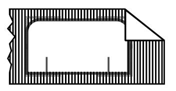
Wrap each package with corrugated board and secure it with tape.
